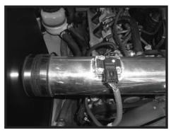
Step 16 Connect the MAF sensor connector by pushing the connector on the sensor.
