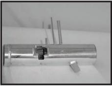
Step 10 Install the factory MAFS on the intake tube using the supplied Phillips head screws.
