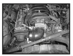
Step 12 Install the coupler over the throttle body and secure with a supplied 3.5" clamp. Install a second clamp but do not tighten at this time.
