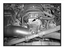
Step 5 Loosen the factory clamp on the throttle body.
