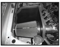
Step 17 Install the filter and securely fasten to the velocity stack adaptor.
