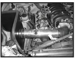
Step 13 Install the intake tube. Once in the desired location and everything fits in place, tighten the clamps.
