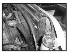
Step 7 Remove the bolt in the radiator shroud. This will be reused in a later step.
