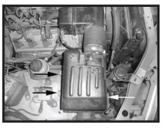
Step 6 Remove the factory air box and tube assembly by removing the three 10mm bolts and lifting it out.
