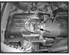
Step 3 Disconnect the Mass Air Flow Sensor (MAFS) connector. Remove the wire loom that is clipped to the factory air box.
