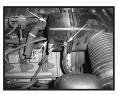
Step 4 Remove the 3 vacuum hoses from the stock air box.
