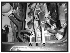
Step 15 Reconnect the 3 vacuum hoses to the correct fitting.
